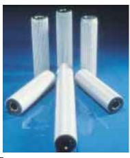
We offer a cost-effective line of low-pressure cartridge filters for a full range of applications, including the filtration of raw materials, additives, intermediates and pre-polymers. Incorporating our DYNALLOY or DYNAMESH media, they are cleanable and reusable and are available in standard lengths of 254 mm, 508 mm, and 762 mm (10", 20" and 30"
